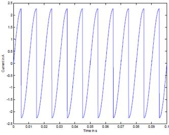
Figure 14: Output Current waveform for 100 Hz
