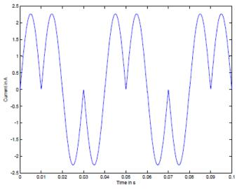
Figure 10: Output Current waveform for 25 Hz
