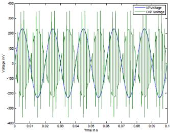
Figure 15: Input and Output Voltage waveform for 500 Hz
