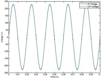
Figure 11: Input and Output Voltage waveform for 50 Hz
